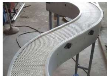
S-bend shaped conveyor
