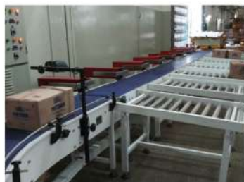
Heavy-duty conveyor with automated sorting
