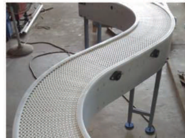
S-bend shaped conveyor
