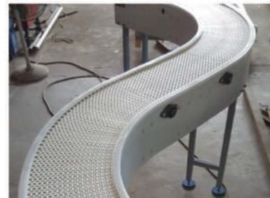
S-bend shaped conveyor
