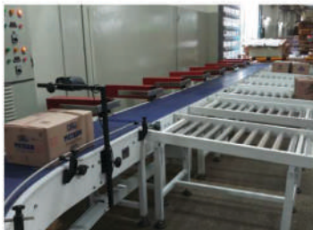
Heavy-duty conveyor with automated sorting
