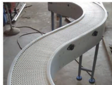
S-bend shaped conveyor
